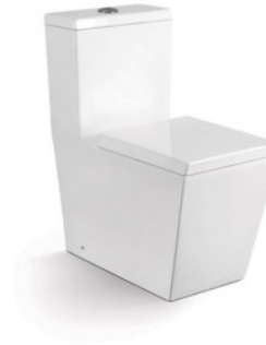
Salacia Two-piece toilet Dos piezas inodoro S-trap 250mm P-trap 180mm Roughing-in
