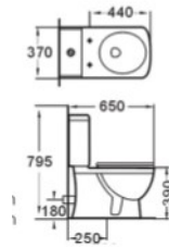
Salacia Two-piece toilet Dos piezas inodoro S-trap 250mm P-trap 180mm Roughing-in
